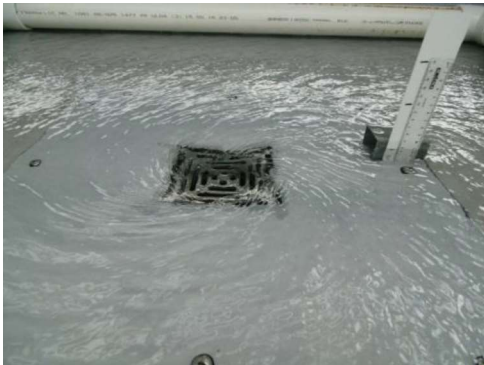
Weir flow - 2 L/s (35mm)
