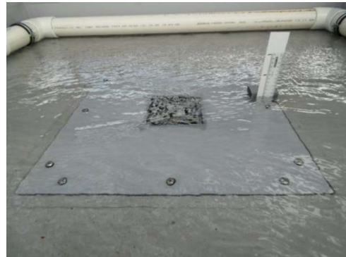
Surcharged flow - 3 L/s (40mm)
