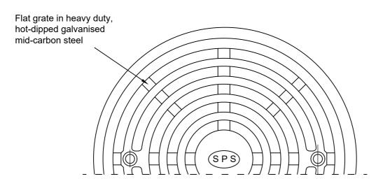
Load-tested to Class D of AS3996-2006
