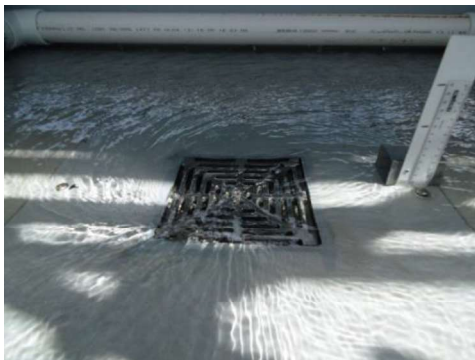
Weir Flow – 4 L/s (25mm)
