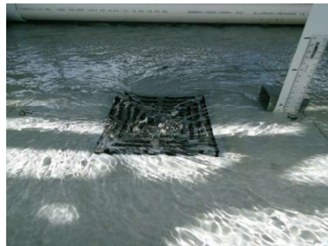
Orifice Flow – 6 L/s (30mm)
