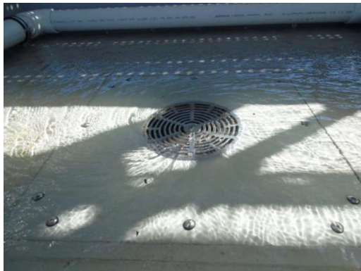
Weir Flow – 2.5 L/s (30mm)
