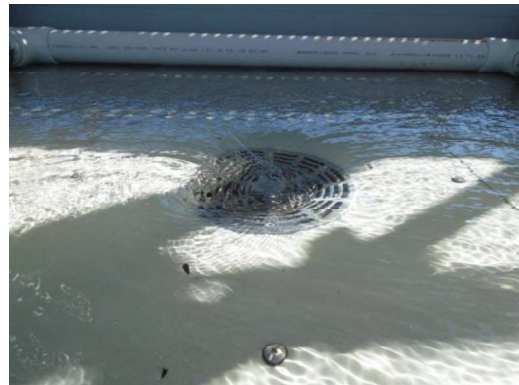
Choked Flow – 6 L/s (42mm)
