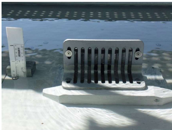
Weir Flow – 2 L/s (50mm)
