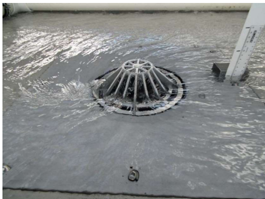
Weir Flow 8 L/s (37mm)
