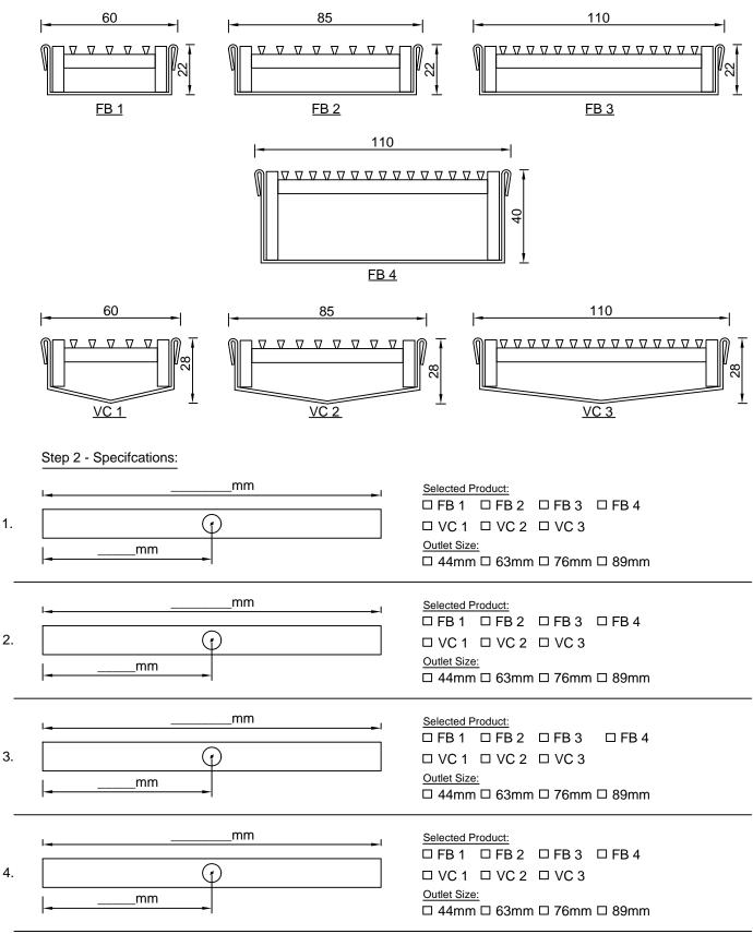
Outlet size must be smaller than width of the channel width; Channel and grates will be 3000mm at maximum, any longer and a joiner will be provide; All 316L SS assembly. Tolerance +/- 1.5mm
