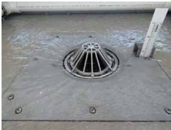
Weir Flow – 1.5 L/s (7mm)
