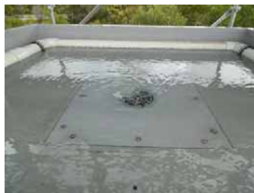
Surcharged flow – 3 L/s (75mm)
