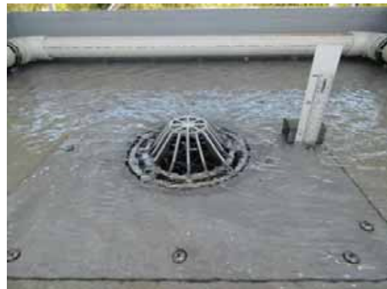
Surcharged Flow 3 L/s (20mm)
