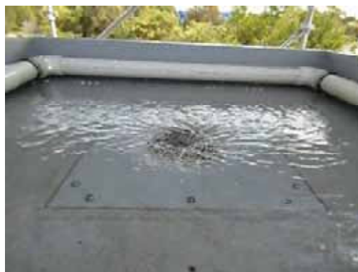
Surcharged flow – 3 L/s (30mm)
