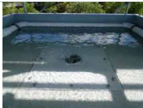
Orifice Flow - 3.0 L/s (80mm)
