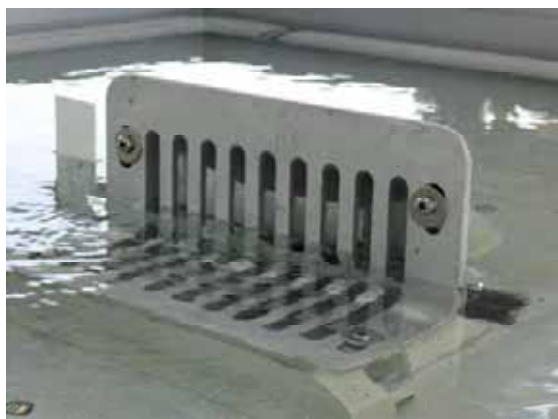
Weir Flow – 4.0 L/s (80mm)
