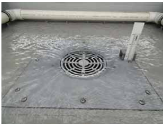
Weir Flow – 3 L/s (15mm)
