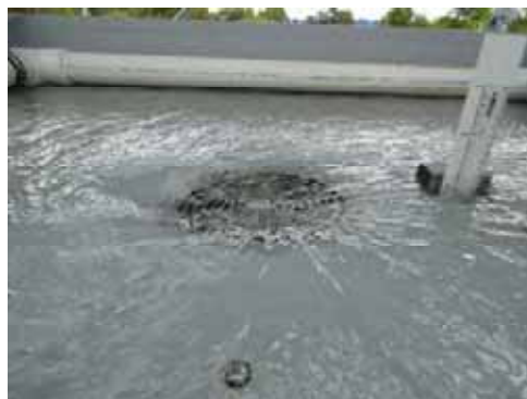
Surcharged Flow – 6 L/s (40mm)
