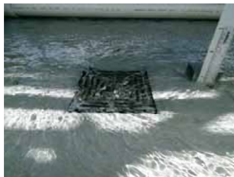
Orifice Flow – 6 L/s (30mm)
