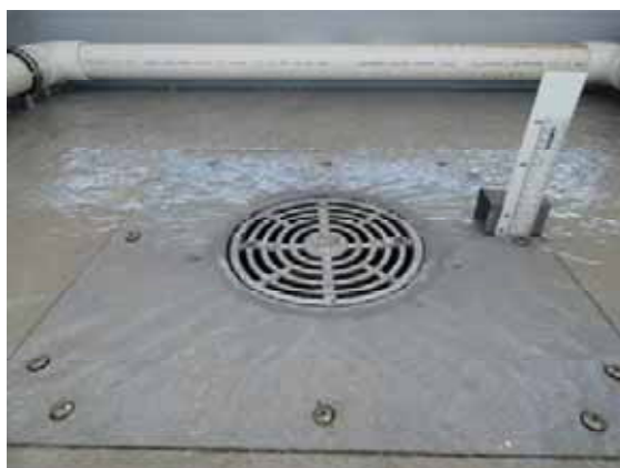
Weir Flow – 1.5 L/s (6mm)
