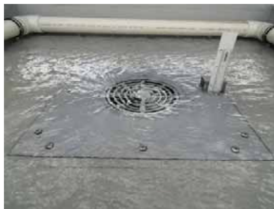
Surcharged flow – 4 L/s (20mm)
