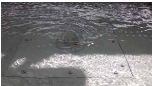
Surcharged Flow - 2.5 L/s (110mm)
