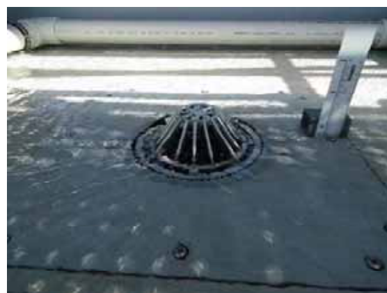
Surcharged flow 5 L/s (30mm)
