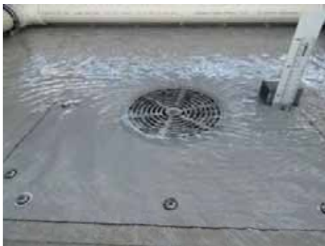
Weir Flow – 2.5 L/s (15mm)
