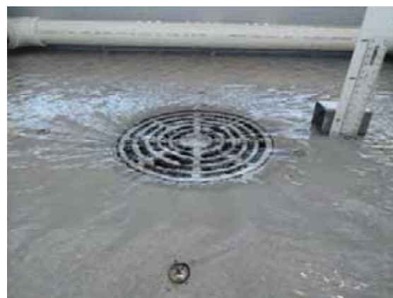
Surcharged Flow – 3 L/s (22mm)
