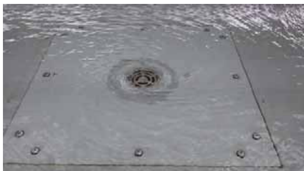
Weir flow - 1.0 L/s (60mm)
