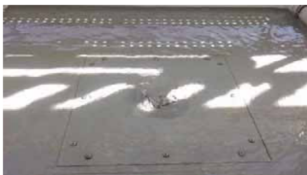
Weir flow - 1 L/s (50mm)
