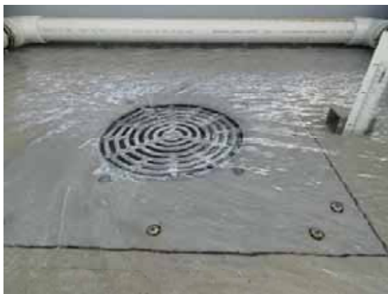
Weir Flow – 7 L/s (25mm)
