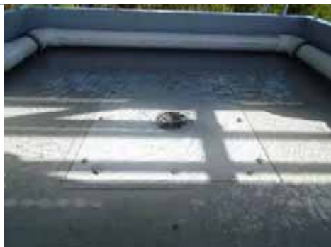
Weir flow - 1 L/s (40mm)
