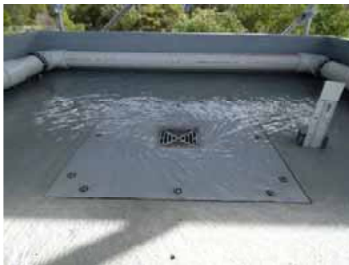
Weir flow - 1 L/s (20mm)
