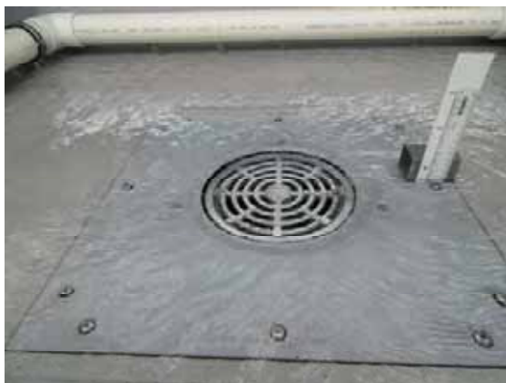
Weir Flow – 3 L/s (13mm)
