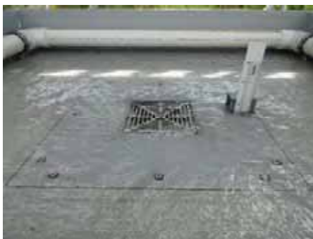
Weir Flow – 2 L/s (20mm)
