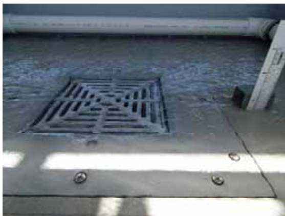
Weir Flow – 7 L/s (18mm)
