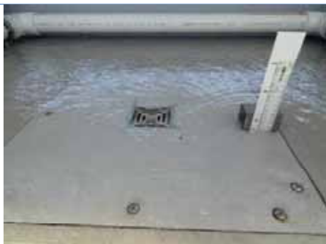
Weir Flow – 0.75 L/s (14 mm)
