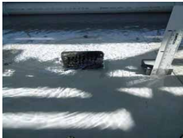
Surcharged Flow – 1 L/s (30mm)
