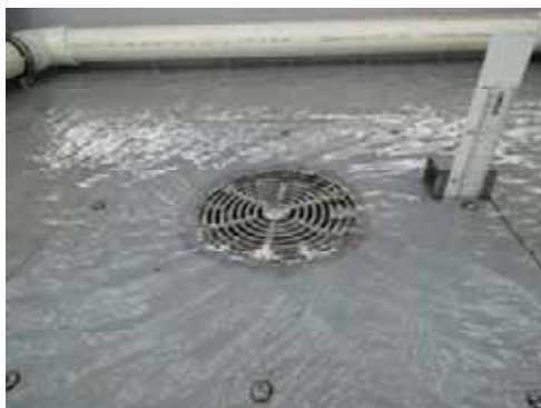
Weir Flow – 2.5 L/s (20mm)
