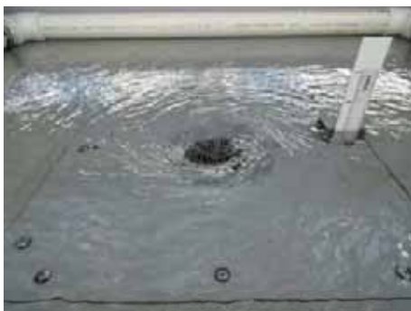
Weir Flow – 2.5 L/s (50mm)
