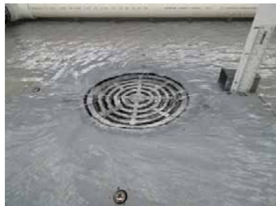
Vortex/surcharged flow 4 L/s (20mm)
