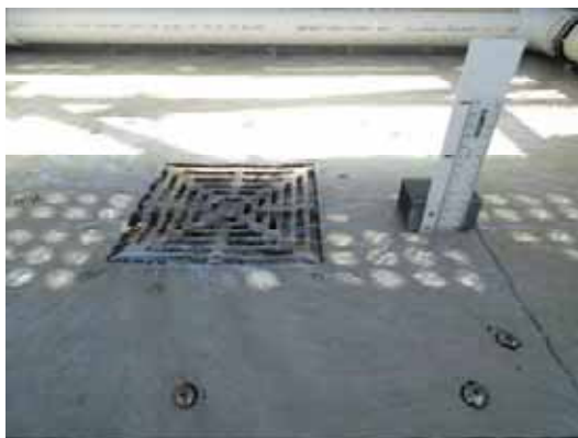
Weir Flow – 6 L/s (18mm)
