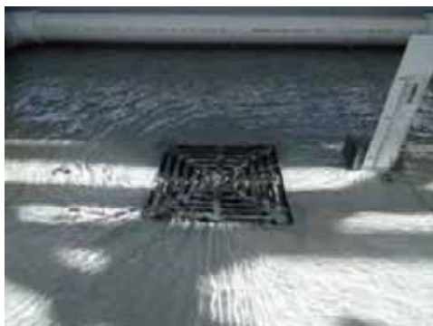
Weir Flow – 4 L/s (25mm)
