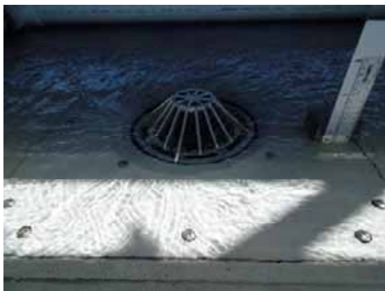
Weir Flow – 8 L/s (30mm)
