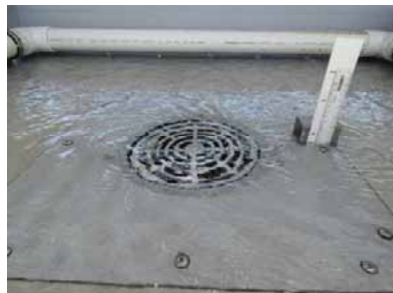
Surcharged Flow – 3 L/s (20mm)
