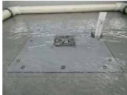
Surcharged flow - 3 L/s (40mm)
