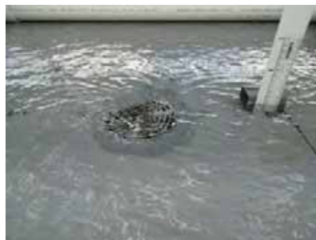
Surcharged flow – 4 L/s (30mm)
