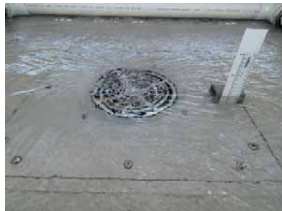
Orifice flow 10 L/s (40mm)
