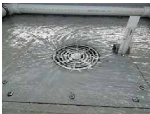
Weir Flow – 7 L/s (30mm)
