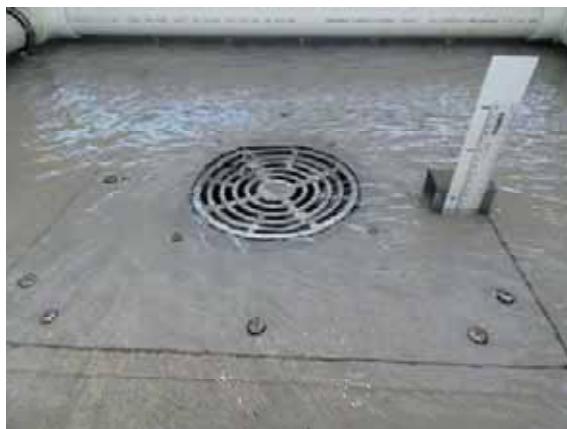
Weir Flow 6.0 L/s (35mm)
