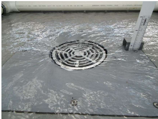
Weir Flow 8 L/s (30mm)
