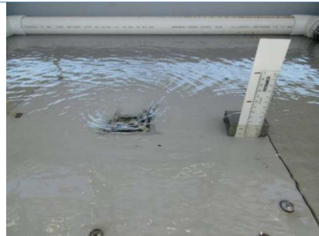
Orifice Flow – 1.5 L/s (50 mm)
