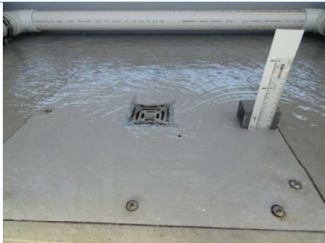
Weir Flow – 0.75 L/s (14 mm)
