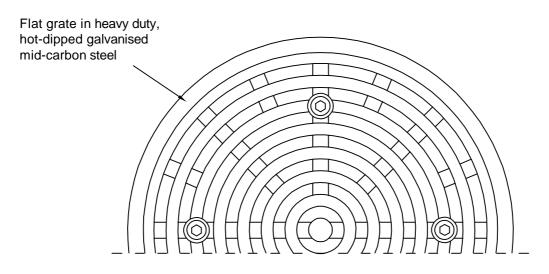
Load-tested to class D of AS3996-2006
