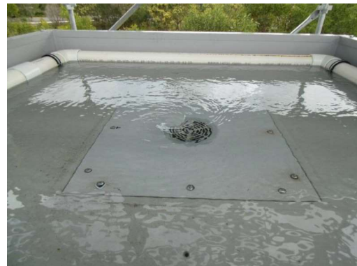
Surcharged flow – 3 L/s (75mm)
