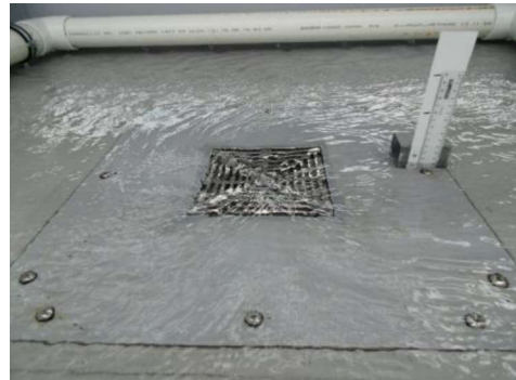
Orifice flow – 4.0 L/s (30mm)
