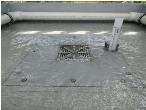
Weir Flow – 2.0 L/s (20mm)
